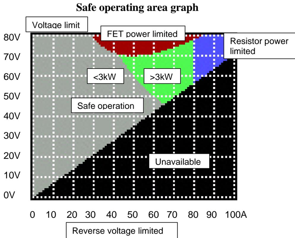
For 35V mode, this graph applies with half the voltage and double the current.
